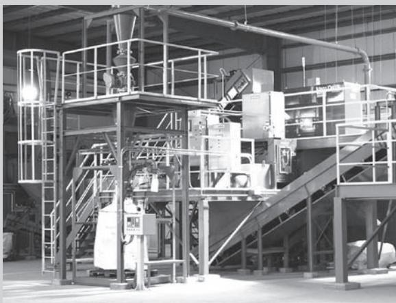
Figure 10. An NRT machine vision and x-ray-based inspection and sorting system installed in a plastics recycling facility located in Nagoya, Japan.
