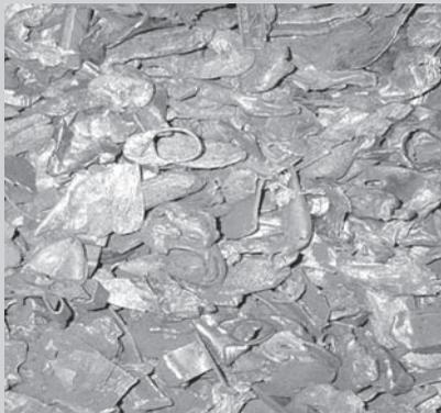
Figure 7. Nonferrous scrap from the separation system, before sortation.
