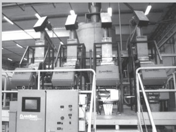
Figure 13. A four-module FlakeSort system installed in a plastics recycling plant in Venice, Italy by NRT.
