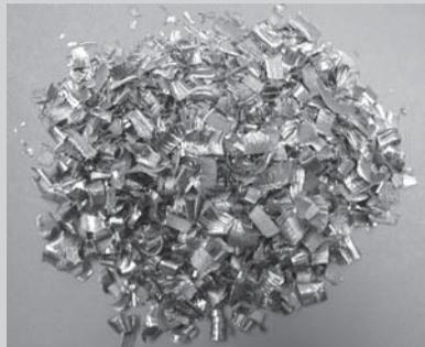
Figure 2. Aerospace metal turnings after shredding.
