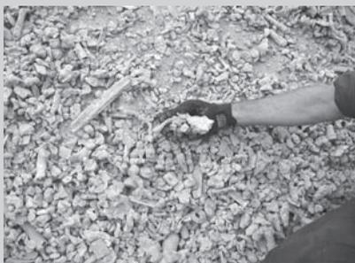
Figure 9. Post-combustion nonferrous concentrates from waste-energy plants can also be sorted using Spectramet technology.
