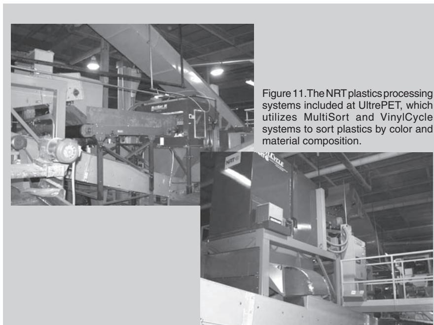
Figure 11. The NRT plastics processing systems included at UltePET, which utilizes MultiSort and VinylCycle systems to sort plastics by color and material composition.
